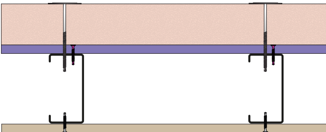
Figure 2 Insulation fixed to studs with typical insulation fixings (Category B in Table 3)
