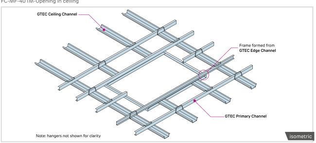
▶ Frames around openings and large penetrations in ceiling to be formed from GTEC Edge Channel with additional GTEC Primary Channel to support opening frame and GTEC Ceiling Channels.
