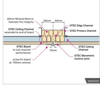
FC-MF-302S-Movement joint - perpendicular to c. channels
