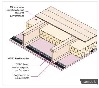
FC-DT-102M-Timber ceiling with resilient bar
