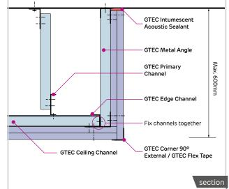
Form 90° junction in ceiling by fixing GTEC Edge Channels at right angle with GTEC Ceiling Channel spanning vertically as required. Hangers to be positioned at maximum 150mm from change in height.
