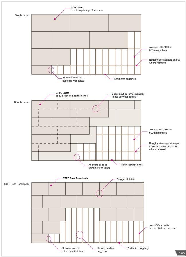
floors and ceilings page 39 of 42 technical services technical.siniat@etexbp.co.uk GTEC Direct-to-Timber Ceiling system is suitable for single, double and multiple layer boarding. Select base layer(s) and finishing layer(s) GTEC Boards by consulting System Performance Tables (pages 3 to 7) and Product Specification see <u>annex b</u>: product reference to achieve required performance. Boards to be supported by joists or intermediate noggings where required.
