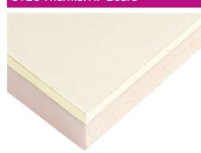
GTEC Standard Board laminated to extruded polystyrene to create a product which offers a significant improvement in insulation over standard plasterboard. 9.5mm plasterboard bonded to extruded polystyrene foam (XPS). (Check building regulations before using in external walls)
