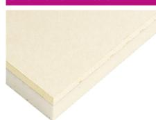
GTEC Thermal PIR Boards are suitable for a wide range of conversion or refurbishment projects requiring significant upgrade to the thermal performance. An additional vapour control layer reduces the risk of condensation. 12.5mm plasterboard bonded to polyisocyanurate foam (PIR). (Check building regulations before using in external walls) Standards: BS EN 13950
