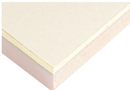
GTEC Standard Board laminated to extruded polystyrene to create a product which offers a significant improvement in insulation over standard plasterboard. 9.5mm plasterboard bonded to extruded polystyrene foam (XPS). (Check building regulations before using in external walls)
