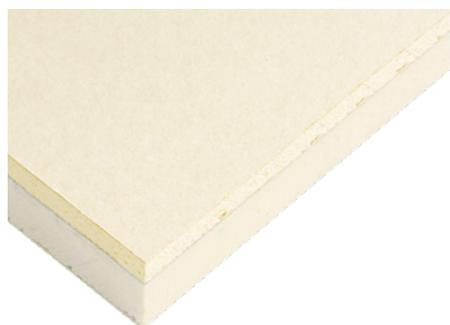
GTEC Thermal PIR Boards are suitable for a wide range of conversion or refurbishment projects requiring significant upgrade to the thermal performance. An additional vapour control layer reduces the risk of condensation. 12.5mm plasterboard bonded to polyisocyanurate foam (PIR). *(Check building regulations before using in external walls)*
